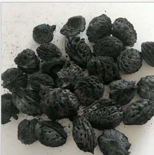
Peach pits are charred in a cast-iron crucible on a wood- and charcoal fire for about 2 hours.
