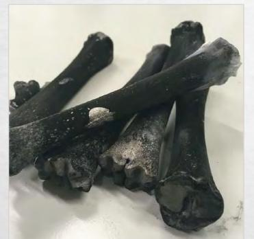
The bones are placed in a crucible which is closed with a lid. The crucible is placed into a fire for 4-5 hours.
